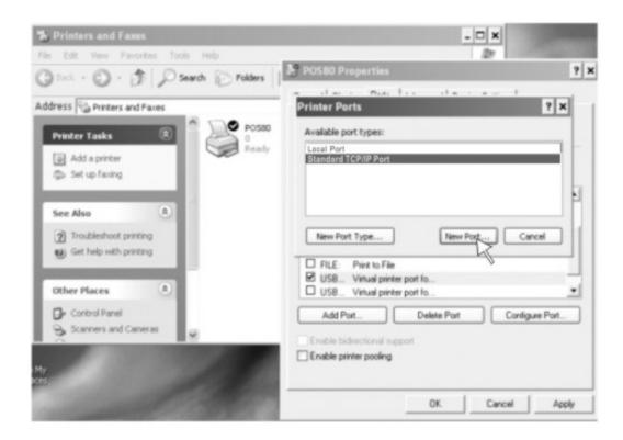
4) according to Add Standard TCP / IP Printer Port Wizard, click Next to continue installation, as shown:
