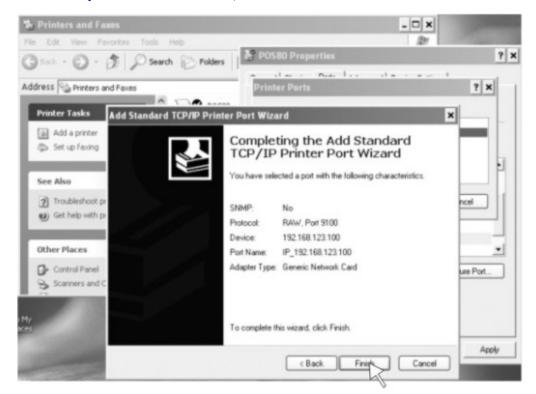
8), according to the printer driver "Properties", click the port, select the correct IP port, click Apply, you can print a test page, as shown:
