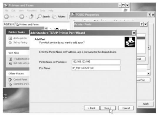
6) according to Add Standard TCP / IP Printer Port Wizard, select the device type --- the standard way, and then click Next to continue installation, as shown:
