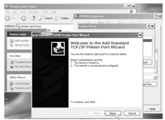
5) according to self-test print of bill IP address enter IP, and then click Next to continue installation, as shown:
