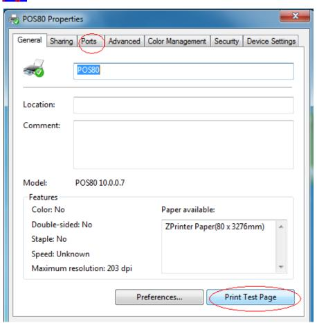
If the printer prints a normal page then it indicates that the driver works successfully. You can use the printer right now, then you don't have to read the content as below.
